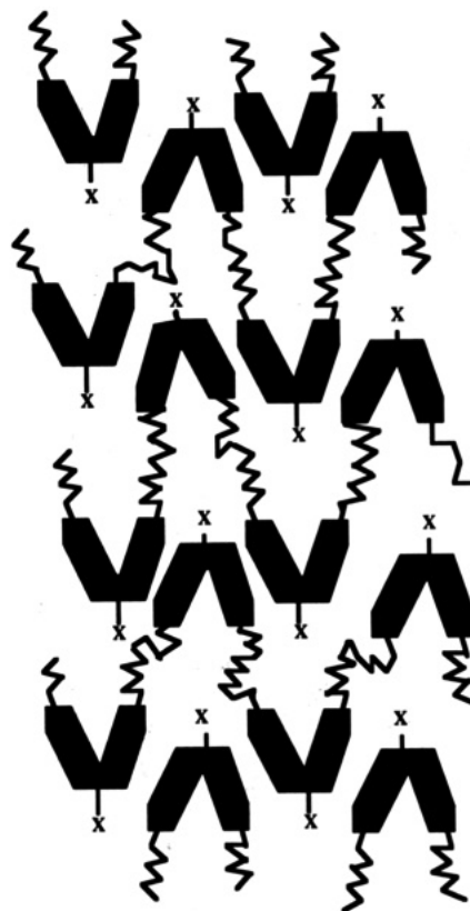
Figure 16. Schematic visualization of the layered structure suggested for P2–P5 smectic mesophases. X = CH 3 , CHO, NO 2 , fused phenyl ring.
